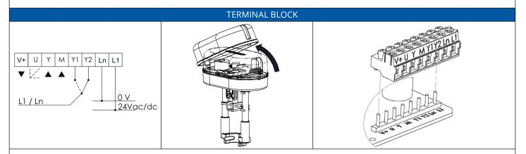
**Note:** To avoid damages to electronic components caused by the PCB bending, do not press too much while fixing the terminal block.
