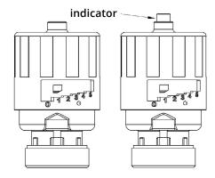
The actuators complete the stroke when the pin exceeds the cover collar by 4mm. O-Ring guarantees IP54 protection with 360° installation position.
