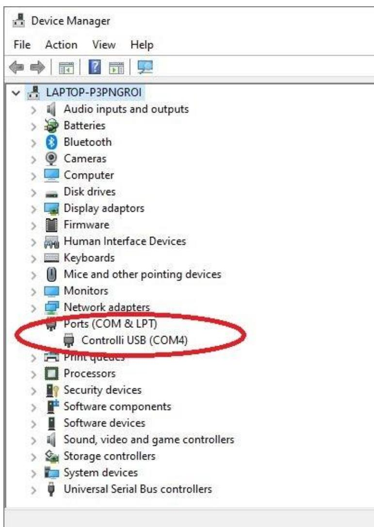
Figure 18. Windows device manager to identify the COM port of the actuator
